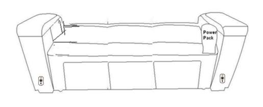
Step2: Slide back receivers into steel mechanism posts in the base of the furniture, and then press both sides of the each back firmly into place to ensure every back automatically locks in place.
